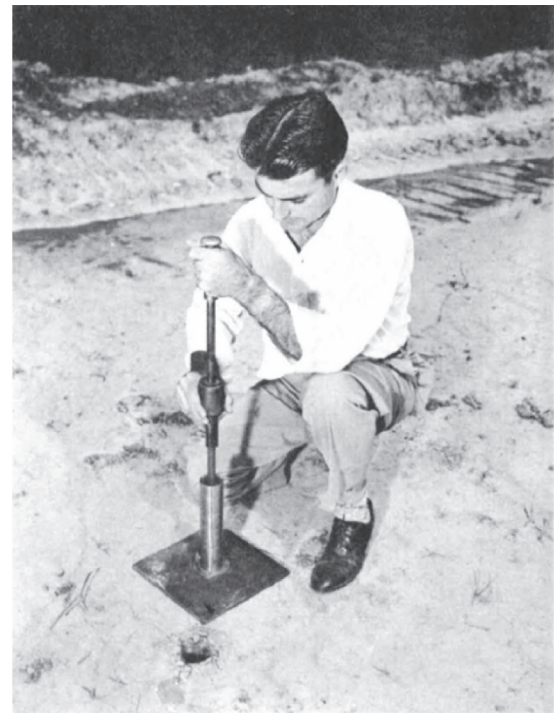
(b) Drop hammer is blowing the soil in the remold cylinder.
