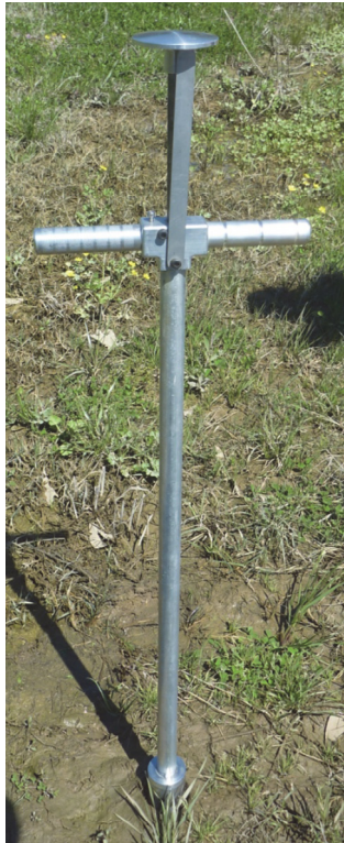
Fig. 39. Hvorslev soil sampler. Reprinted from (Stevens et al., 2013) with permission of US Army Engineer Research & Development Center.
