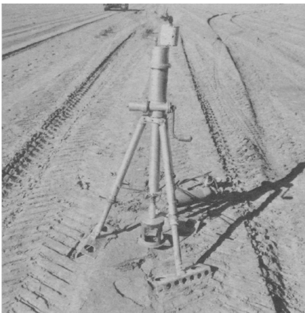
Fig. 30. Shear test device of a portable bevameter. Reprinted from (Rula and Nuttall, 1971) with permission of US Army Engineer Research & Development Center.
