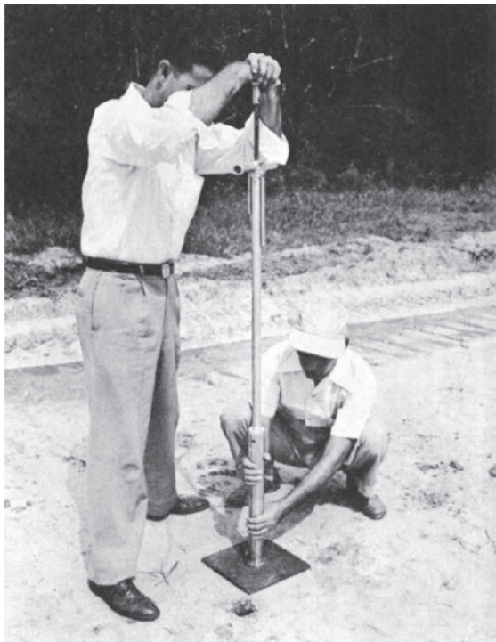
(a) Soil is transported from the Hvorslev sampler to the remold cylinder.
