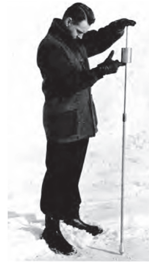
(b) Rammsonde penetrometer in use. Reprinted from (Ueda et al., 1975) with permission of U.S. Army Cold Regions Research and Engineering Laboratory.
