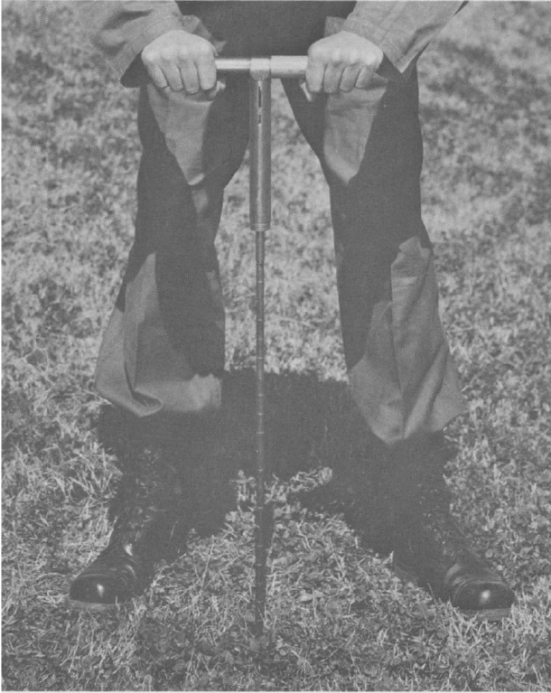
Fig. 29. Airfield penetrometer in use. Reprinted from (Burns and Carr, 1965) with permission of US Army Engineer Research & Development Center.
