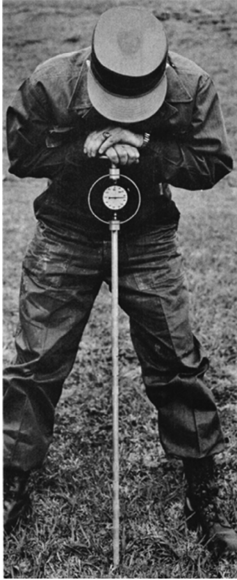
Fig. 34. A WES cone penetrometer in use. A dial indicator displays the reading of the penetration resistance. Reprinted from (Mobility and Environmental Systems Laboratory (U.S.), 1957) with permission of US Army Engineer Research & Development Center.
